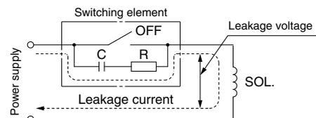
AC/Class B built-in full-wave rectifier coil: 10% or less of rated voltage
