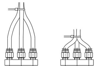
Fig. 2 Binding tubes with bands
