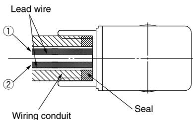
(Connection G1/2 Tightening torque of 0.5 to 0.6 N·m)
