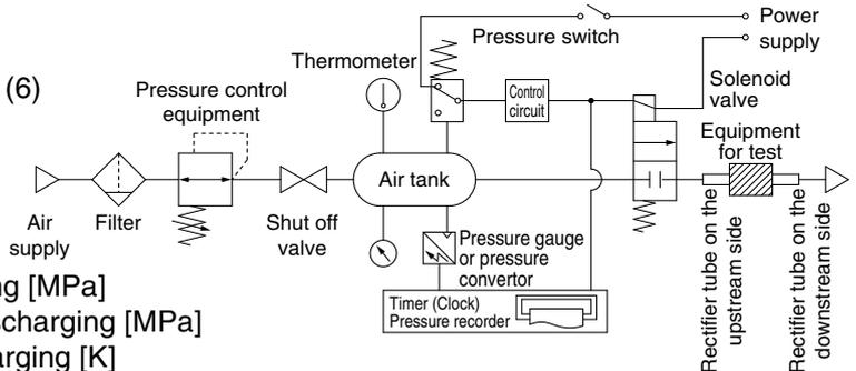
Fig. (2) Test circuit based on JIS B 8390
