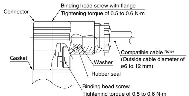
Note) For an outside cable diameter of  $\phi 9$  to 12 mm, remove the internal parts of the rubber seal before using.
